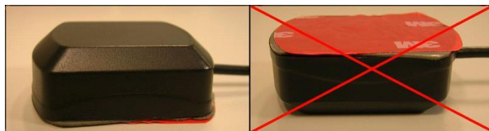
Figure 37. Correct GPS antenna mounting
